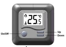
Hold the icon O button (above Figure) for 3 second – to turn on or off the thermostat.
